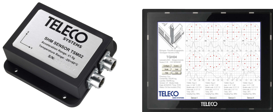
Figure 1: SHM602 system: (a) sensing units TSM02 and (b) data acquisition and storage controller TSD10
