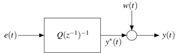
Figure 2. Structure of AR+noise models
