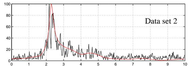
Figure 12. Power spectra of  $y_2$ ; measures and model (red)
