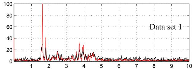
Figure 19. Power spectra of  $y_2$ : measures from MEMS-based (black) and piezoelectric accelerometers (red)
