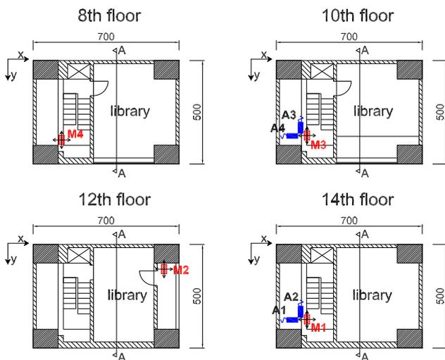
Figure 6. Accelerometer locations in the selected floors
