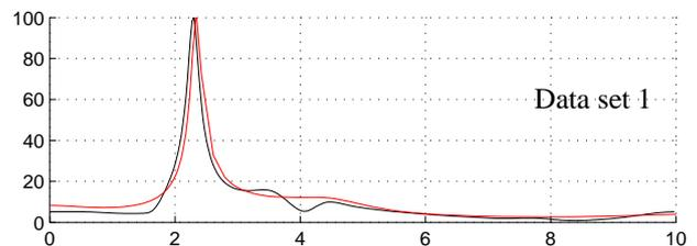
Figure 20. Power spectra of  $y_2$ : ident. models obtained from MEMS-based (black) and piezoelectric accelerometers (red)
