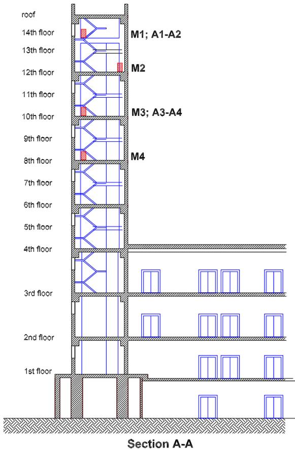
Figure 5. Accelerometer locations in the tower
