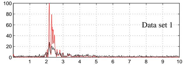
Figure 18. Power spectra of  $y_1$ : measures from MEMS-based (black) and piezoelectric accelerometers (red)
