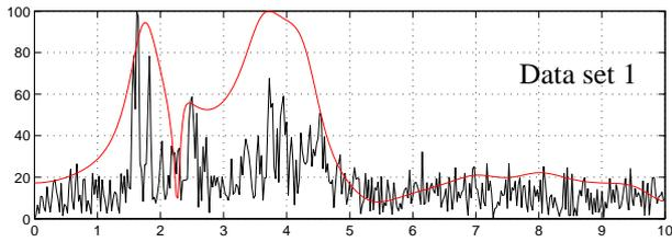
Figure 7. Power spectra of  $y_1$ ; measures and model (red)
