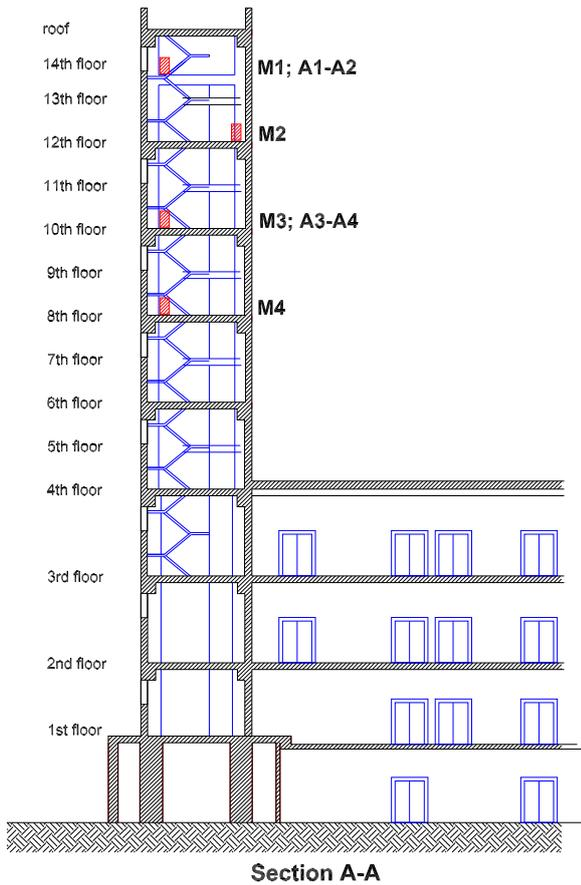
Figure 5. Accelerometer locations in the tower
