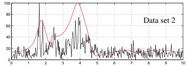
Figure 11. Power spectra of  $y_1$ ; measures and model (red)
